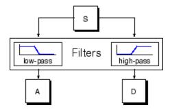
The original signal, S, passes through two complementary filters and emerges as two signals.
