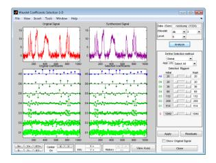
The tool displays below the original signal (on the left) its wavelet decomposition: the approximation coefficients A6 and detail coefficients from D6 at the top to D1 at the bottom. In the middle of the window, below the synthesized signal (which at this step is the same, since all the wavelet coefficients are kept) it displays the selected coefficients.
