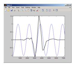
Recall that the CWT coefficients are obtained by computing the product of the signal with the shifted and scaled analyzing wavelet and integrating the result. The following figure shows the product of the wavelet and the sinusoid from the preceding figure.
