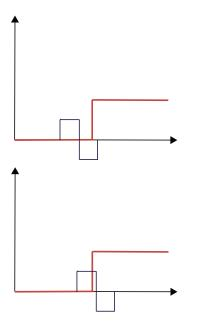
In the top figure, the wavelet has just begun to overlap with the unity portion of the unit step. In this case, the CWT coefficients are negative, but not as large in absolute value as those obtained at position B. In the bottom figure, the wavelet has shifted past position B and the positive deflection of the wavelet begins to contribute to the integral. The CWT coefficients are still negative, but not as large in absolute value as those obtained at position B.
