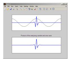
The product shown in the bottom pane closely resembles the analyzing wavelet. Integrating this product results in a CWT coefficient near zero.
