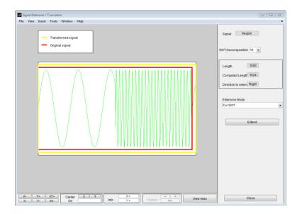
Since the signal is of length 1000 and the decomposition level needed for SWT is 10, the tool performs a minimal right periodic extension. The extended signal is of length 1024.
