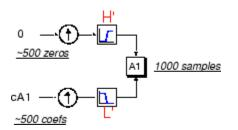
The process yields a reconstructed *approximation* A1, which has the same length as the original signal S and which is a real approximation of it.
