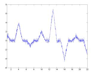
In this case, the wavelet coefficients should remove a first-order polynomial. If the signal value at an odd index, x(2n+1), is well approximated by a first-order polynomial fitted to the surrounding sample values, then 1/2(x(2n)+x(2n+2)) should provide a good fit for x(2n + 1). In other words, x(2n+1) should be the midpoint between x(2n) and x(2n+2).
