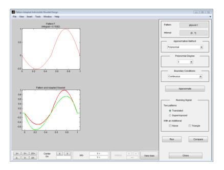
After a pause for computation, the tool displays the new wavelet in green superimposed with the original pattern in red.
