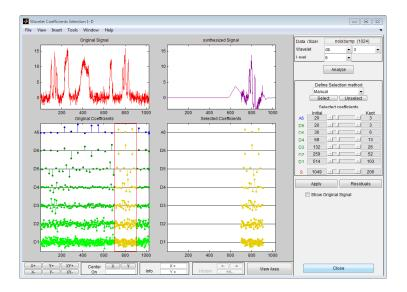
This illustrates that wavelet analysis is a local analysis since the signal is perfectly reconstructed around the position 800. Check the **Show Original Signal** to magnify it.
