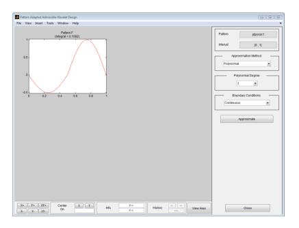
The selected pattern denoted by F is defined on the interval [0,1] and is of integral 0.1592. It is not a wavelet, but it is a good candidate because it oscillates like a wavelet.
