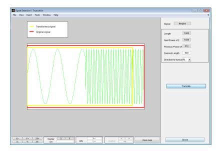
The tool displays the original signal delimited by a red box and the truncated signal delimited by a yellow box. The signal has been truncated by deleting 100 values on the right side.
