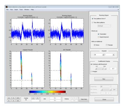
This tool displays the pattern detection performed with the adapted wavelet on the left and db1 wavelet (default) on the right. The two positions are perfectly detected in both cases but scales are slightly underestimated by the db1 wavelet.
