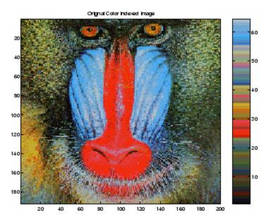
The color bar to the right of the image is not smooth and does not monotonically progress from dark to light. This type of indexed image is not suitable for direct wavelet decomposition with the toolbox and needs to be preprocessed.
