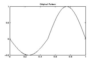
% To synthesize a new wavelet adapted to the given pattern, use % a least squares polynomial approximation of degree 6 with % constraints of continuity at the beginning and the end of the % pattern. [psi,xval,nc] = pat2cwav(Y, 'polynomial',6, 'continuous');
