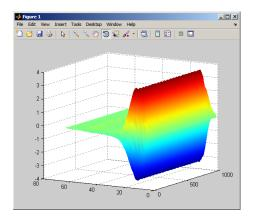
The final example constructs a signal consisting of both abrupt transitions and smooth oscillations. The signal is a 2-Hz sinusoid with two introduced discontinuities.
