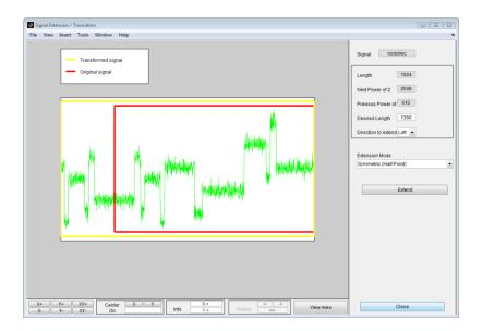
The tool displays the original signal delimited by a red box and the transformed signal delimited by a yellow box. The signal has been extended by left symmetric boundary values replication.
